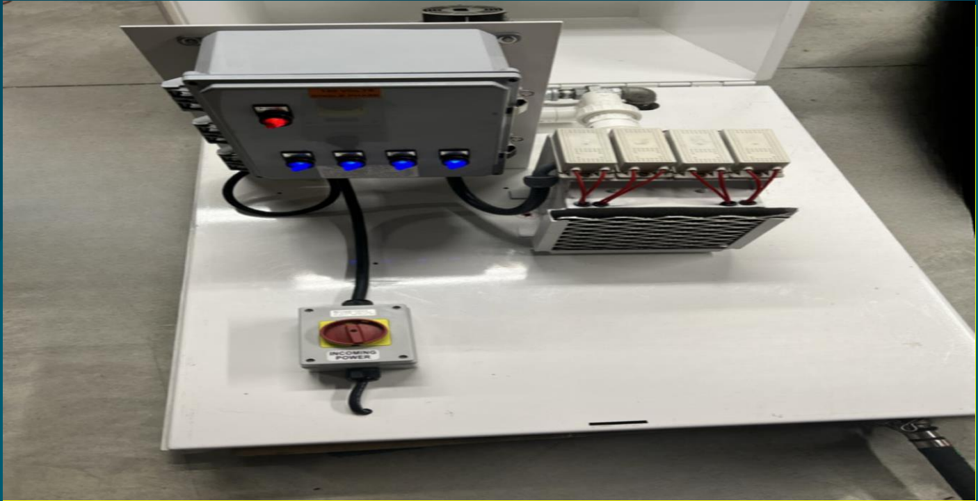
Picture: Demo Blower and O3 manifold for industrial water
