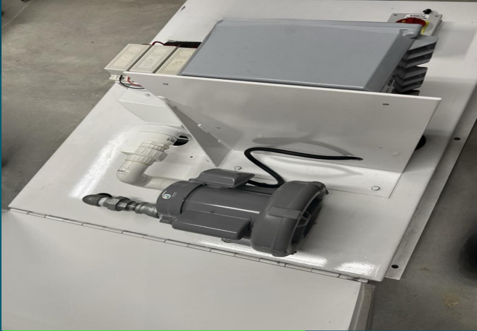
Picture: Kleen 03 manifold,blower,and controls Top view
