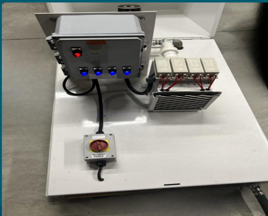
Picture: Kleen O 3 Ozone Manifold and control's Front view
